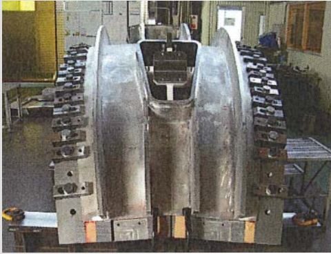
Welded port stub & ribs
