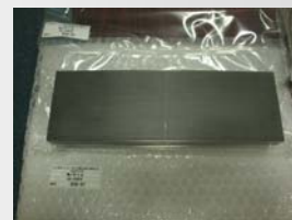
CFC (type I) material for bolted CFC tiles (part 2)
