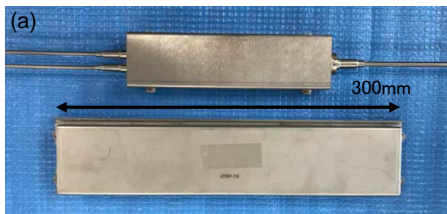
Figure 1: External view of junction boxes (upper: new, lower: original)
