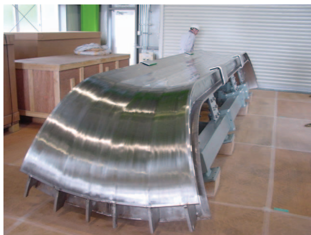
Inboard segment of 40° sector on assembly jig in VV sector assembly bldg.
