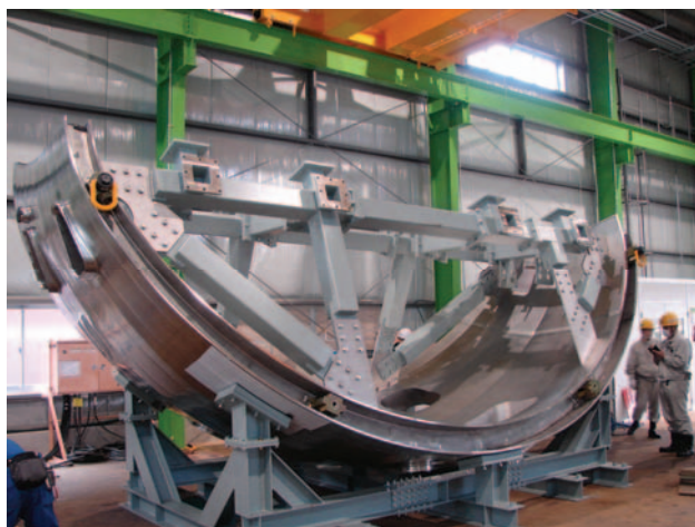
Outboard segment on assembly jig in VV sector assembly bldg.
