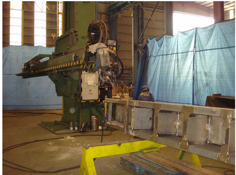
Left: Full penetration welding performed by submerged arc welding process in a side plate of the first U beam profile of the cryostat base lower structure Right: Submerged arc welding machine and first U beam profile of the cryostat base lower structure
