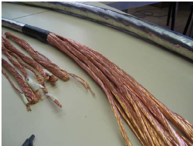
Samples extracted from ICAS internal Cu dummy, aiming at production machines tuning
