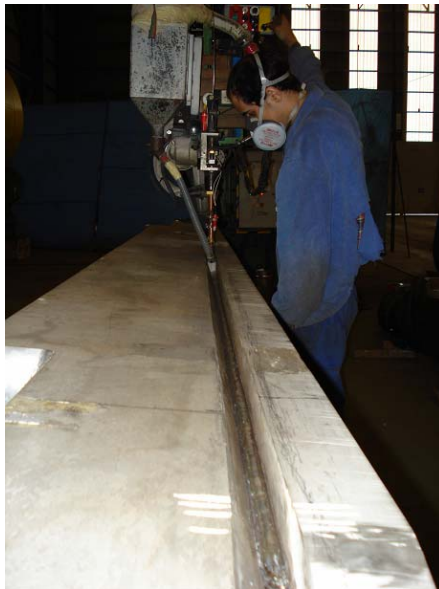
Left: Full penetration welding performed by submerged arc welding process in a side plate of the first U beam profile of the cryostat base lower structure Right: Submerged arc welding machine and first U beam profile of the cryostat base lower structure
