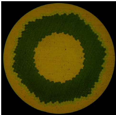
Cross-section of first full-size NbTi strand made from the billet produced by FEC
