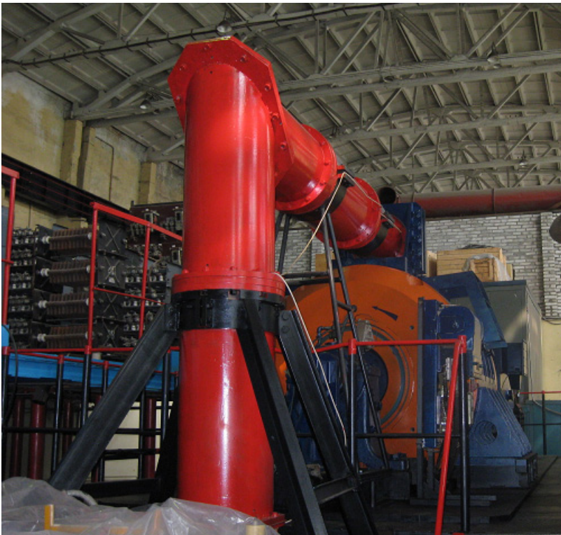
Figure 2 – The homopolar generator able to supply current up to 0.5 MA, developed in the NII EFA laboratory
