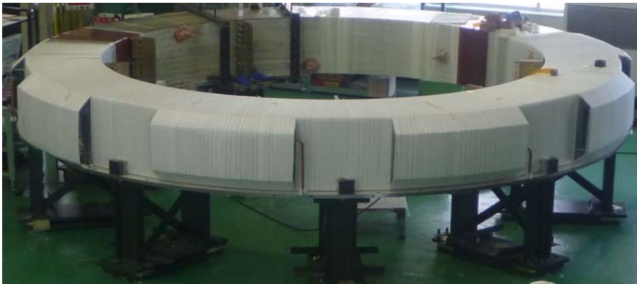
Equilibrium field coil No.4 completed (before hardening)
