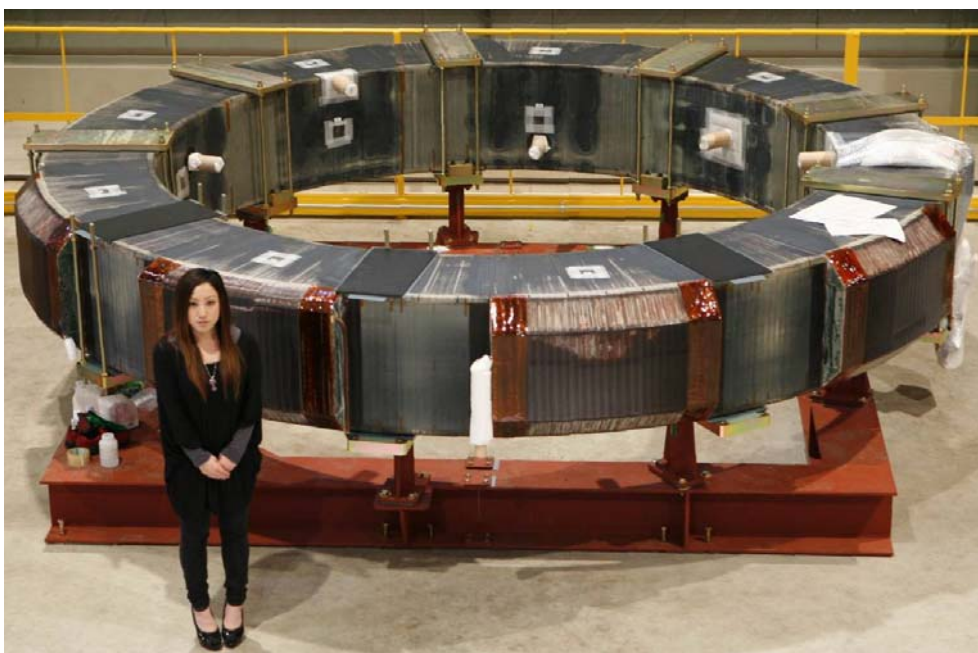
Equilibrium field coil No.4 in the factory before final insulation wrap
