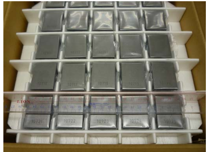
CFC material for mono-block targets
