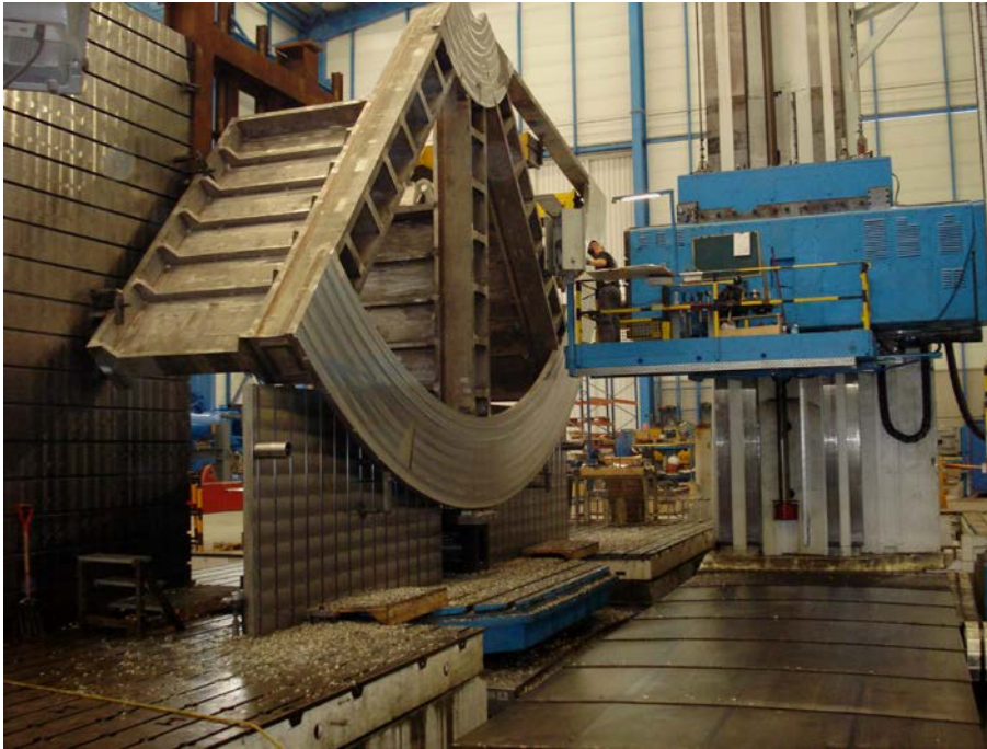
Machining of a lower structure sector
