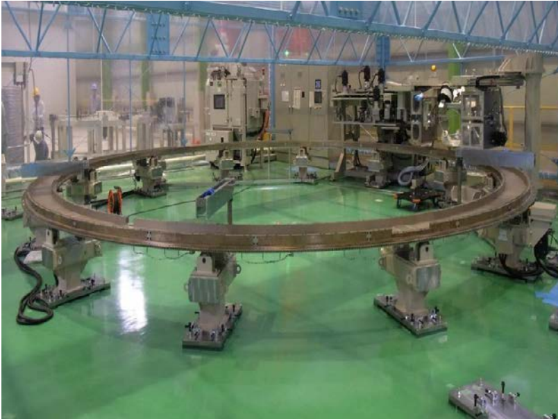
Winding machine set up in the superconducting coil winding building
