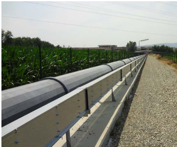
Figure 4: Jacketing lines with 300-metre-long and rectangle shape for JT-60SA and with 800-metre-long and domed shape for ITER at Criotec
