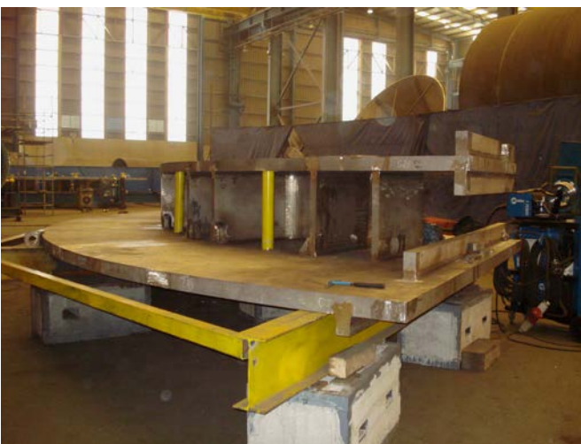
Welding of a double ring sector
