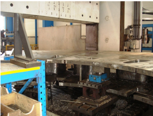
Figure 2: First sector of the double ring being machined
