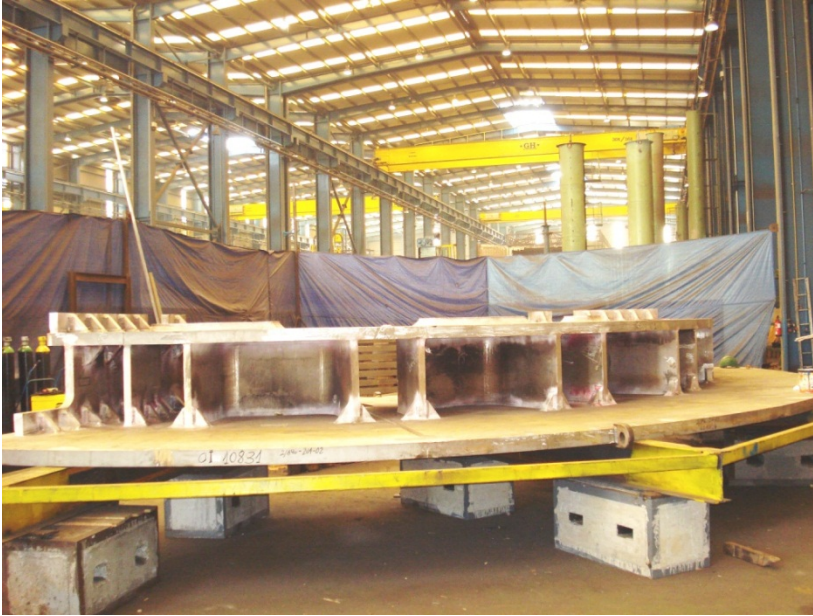
Figure 1: Third sector of the double ring completely welded
