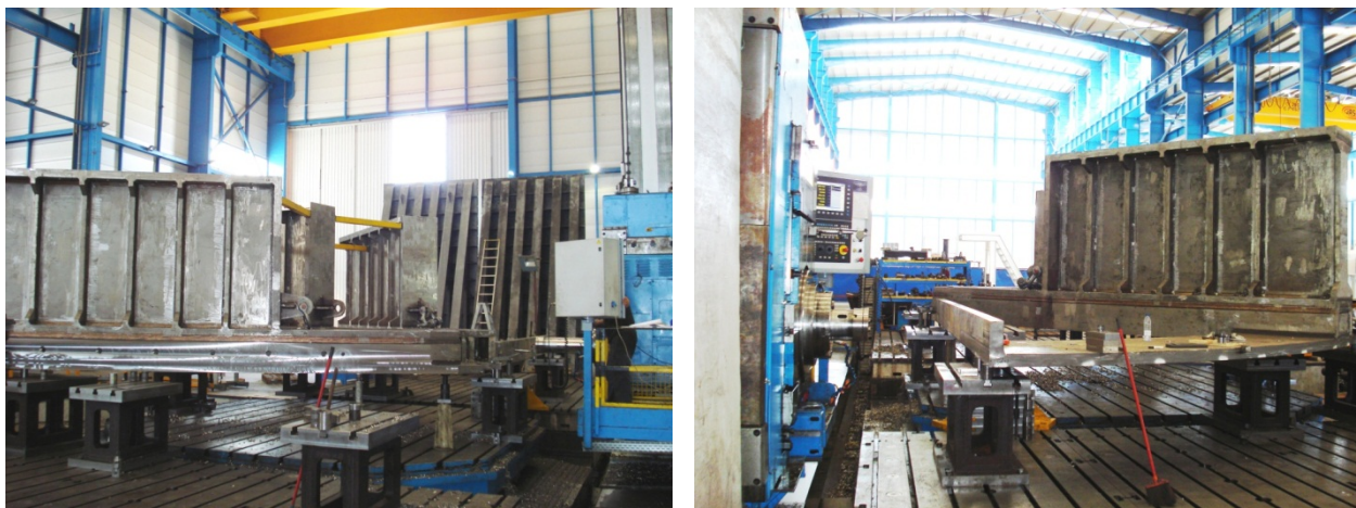
Figure 3: Lower structure sector in the last machining stage
