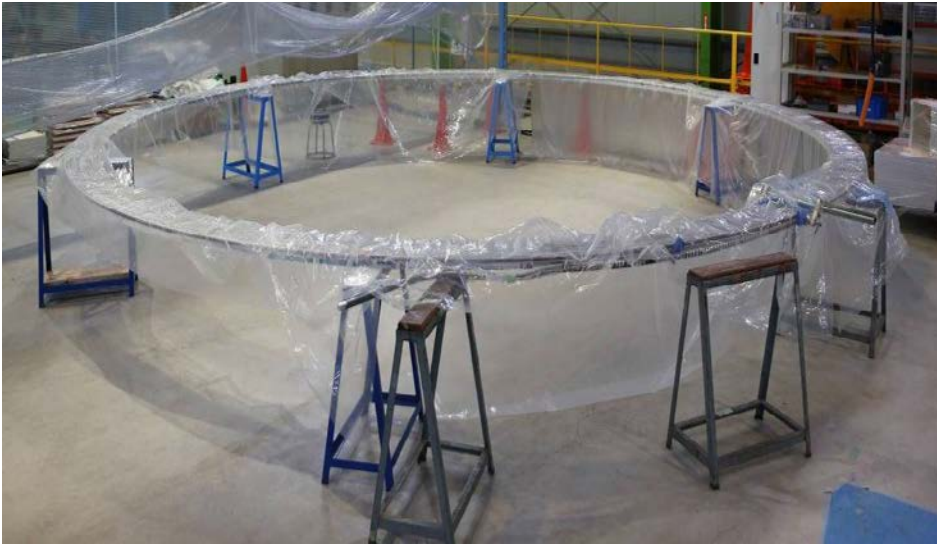
Dummy pancake of the equilibrium field coil No.5
