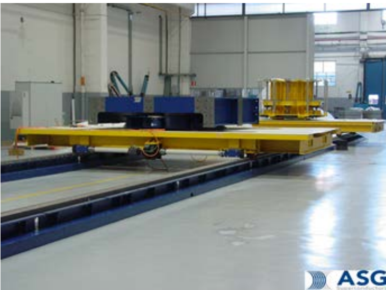
Figure 1: De-spooling and movement/rotating table tools on their carriage before assembly on the winding line rails
