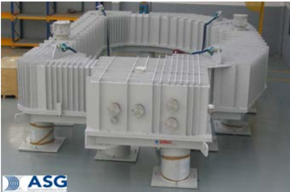
Figure 3: Vacuum chamber for DP and TF coil winding final pressure, leak and electrical tests
