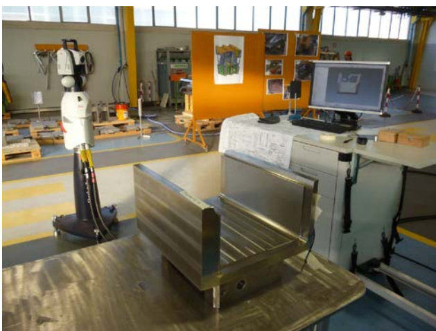
Figure 2: Curved leg mock-up during dimensional survey
