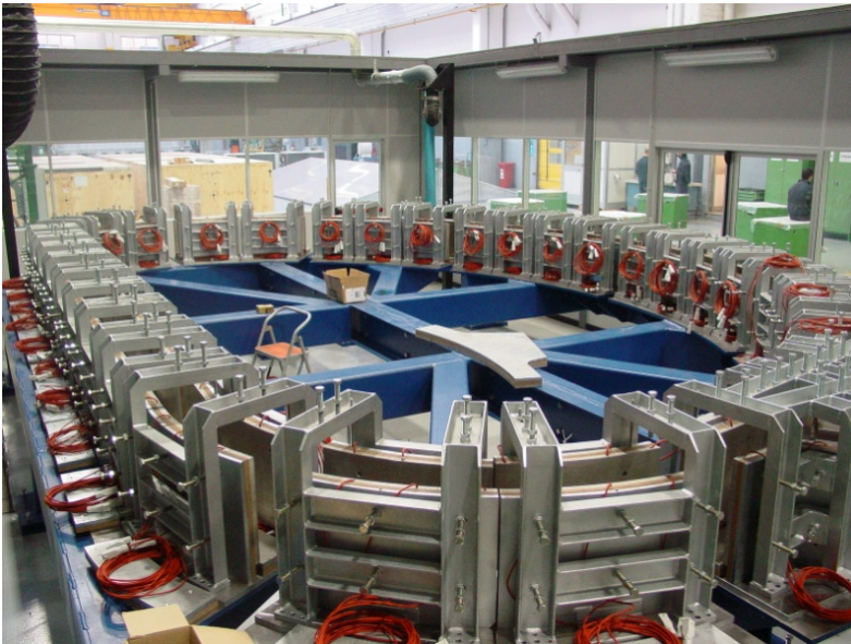
Figure 2: Impregnation mould with resistors already installed
