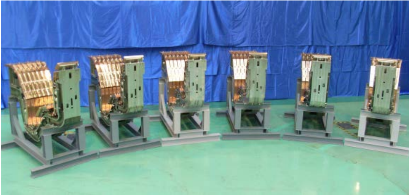
Figure 1: Divertor cassette structures
