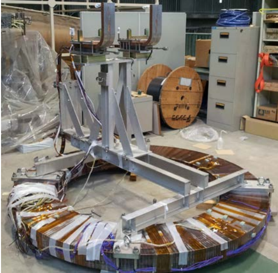
Figure 1: CS model coil before installation
