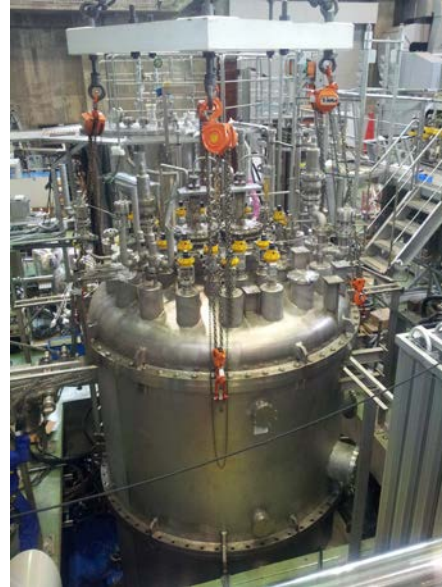
Figure 2: Cryostat for testing the CS model coil at NIFS
