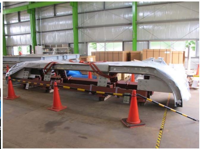
Figure 2: Inboard segment stored in the VV assembly building
