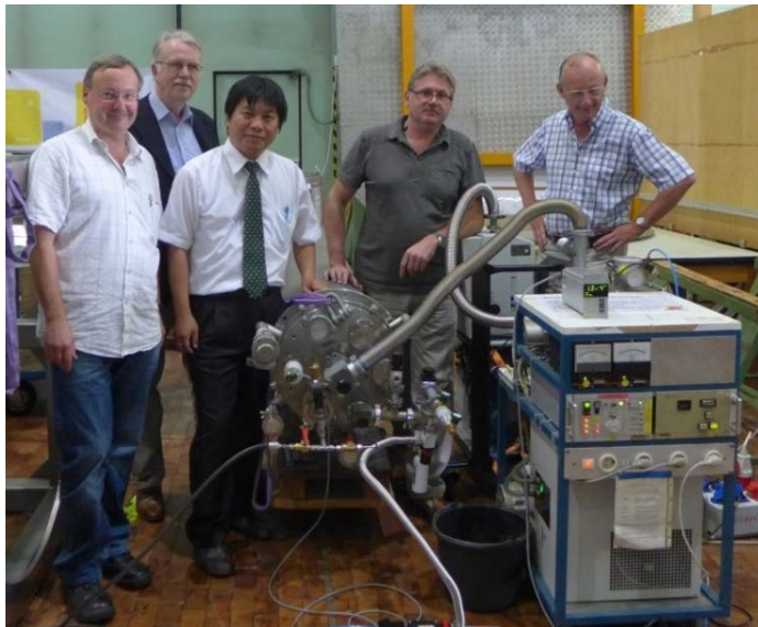
Figure 1: Installation for pressure testing of the HTS CL
