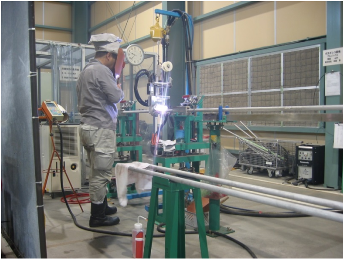
Jacket tube being welded at the Naka site
