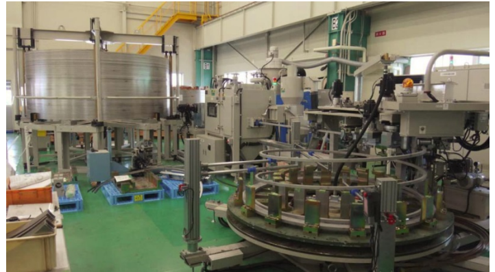
Figure 2: Winding of first OP for JT-60SA CS
