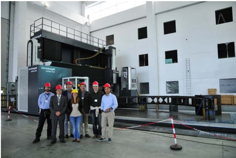
Curved "Spider" jig for TFC casings with the PL, ENEA, F4E and Walter Tosto SpA representatives
