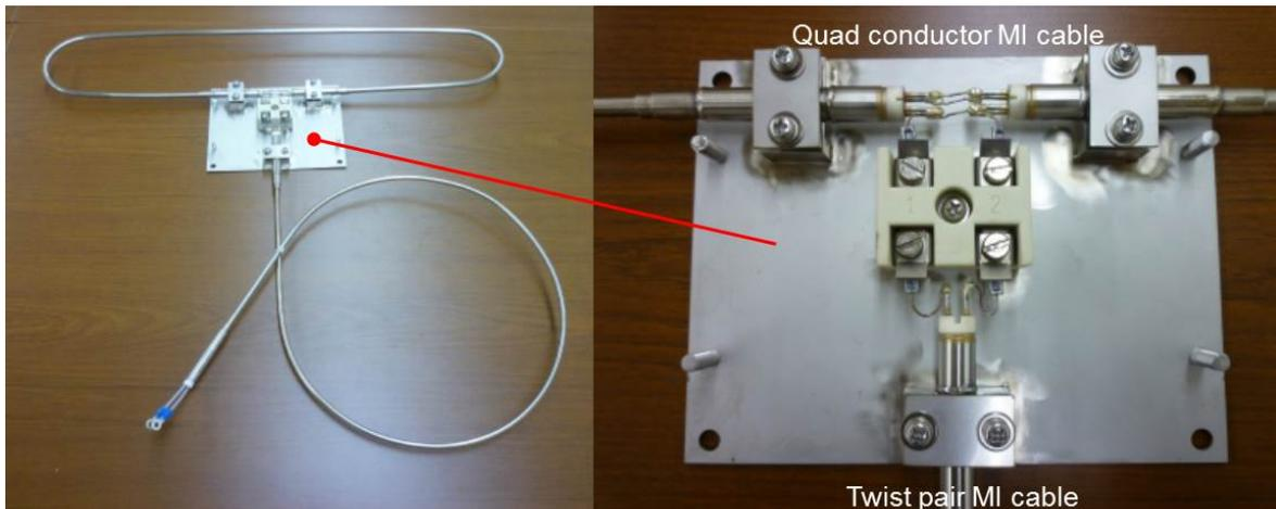
Prototypes of a diamagnetic loop (left) and the joint part (right)
