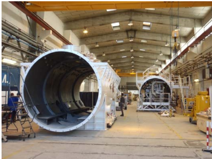
Figure 1: ACB (left) and RCB (right), with the main heat exchanger block integrated, in the AL-AT workshop
