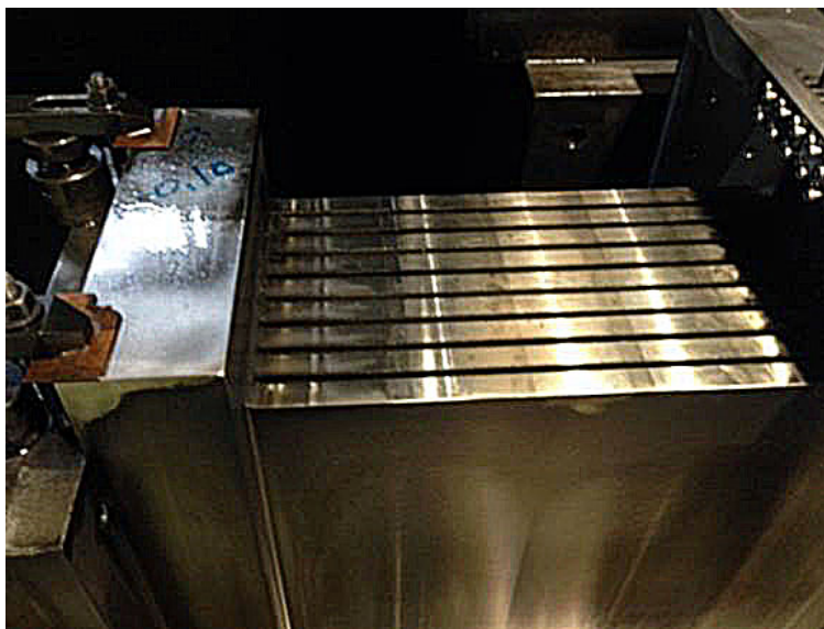
Figure 2: Electrical discharge machined spring plate
