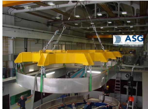
Figure 4: WP moved to cleaning and finishing station
