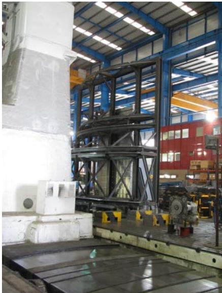
Figure 1: Machining of the welding frame for lower sectors
