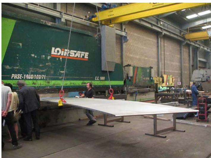
Figure 3: Forming of the first conical part
