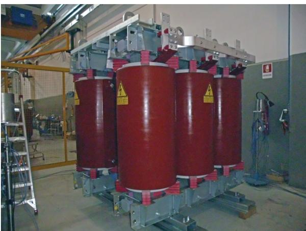
SEA Laboratories, the FPPCC PS transformer tested
