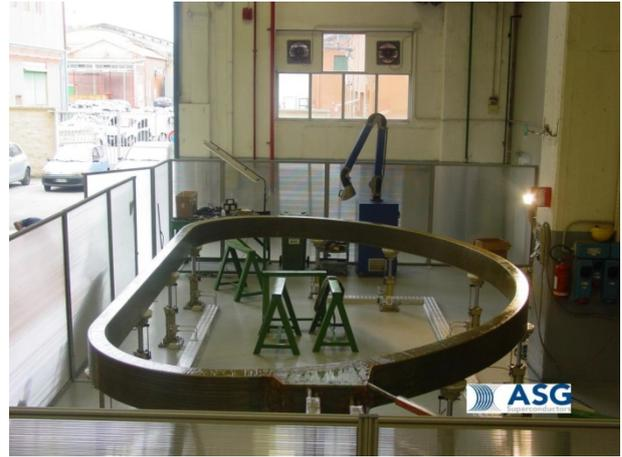
Figure 6: WP waiting for the application of the conductive paint
