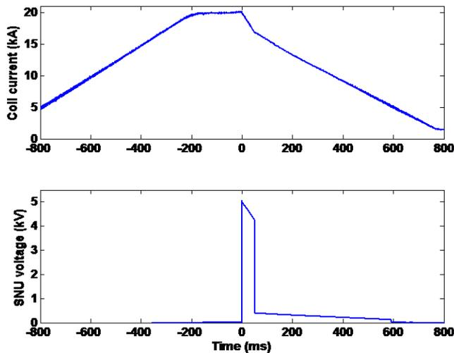
Figure 6: SNU current and voltage measured during a full current and full voltage test in ENEA
