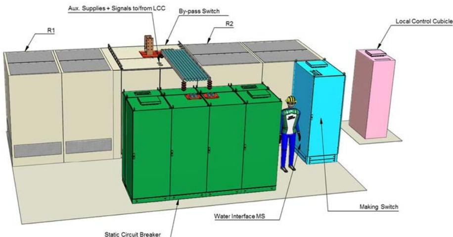
Figure 1: SNU final configuration and layout
