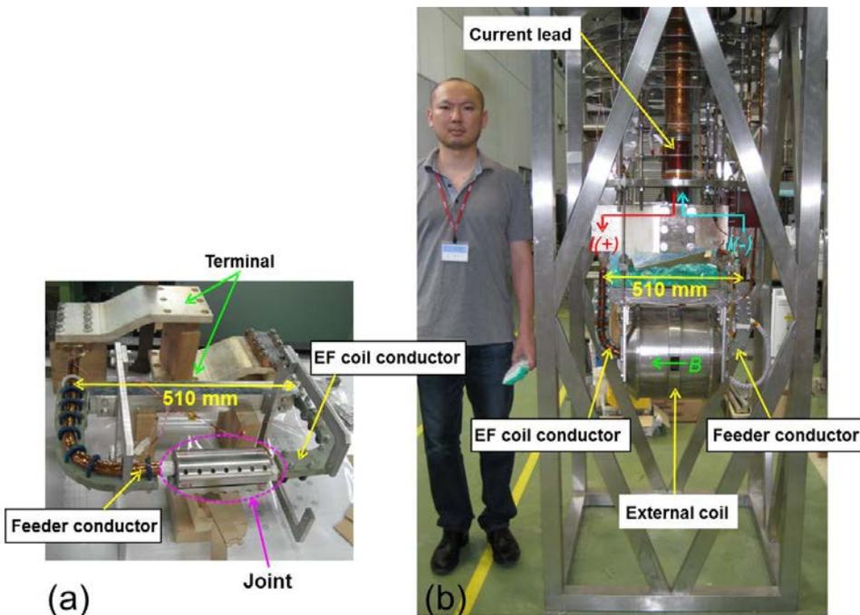
(a) connector prototype of feeder conductor and (b) its installation in the prototype superconducting coil for test
