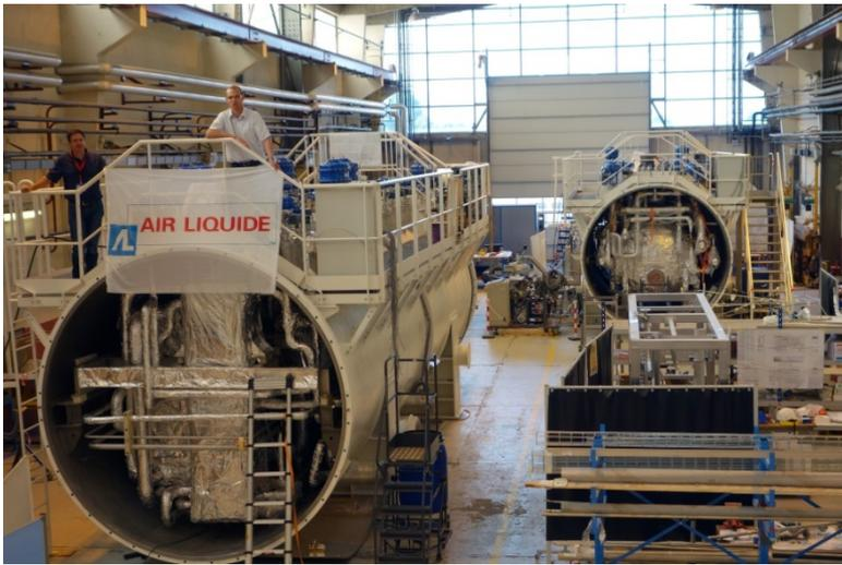
Figure 2: Refrigeration cold boxes (cold end) with insulated cold components
