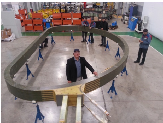
Coil No. 10 after first impregnation
