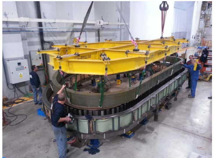
Coil No. 10 extraction from the impregnation mould
