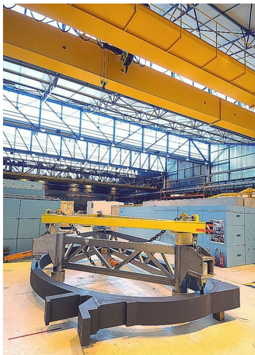
Scale 1 TFC mockup on a CTF test frame
