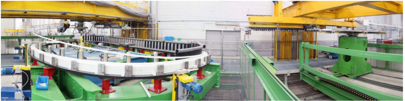
Coil No. 12 winding in progress
