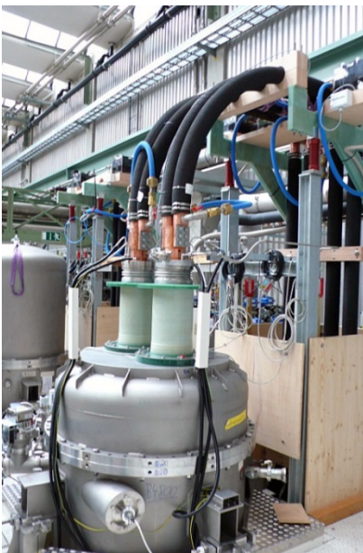
Two TF coil current leads installed in the test facility CuLTka at KIT
