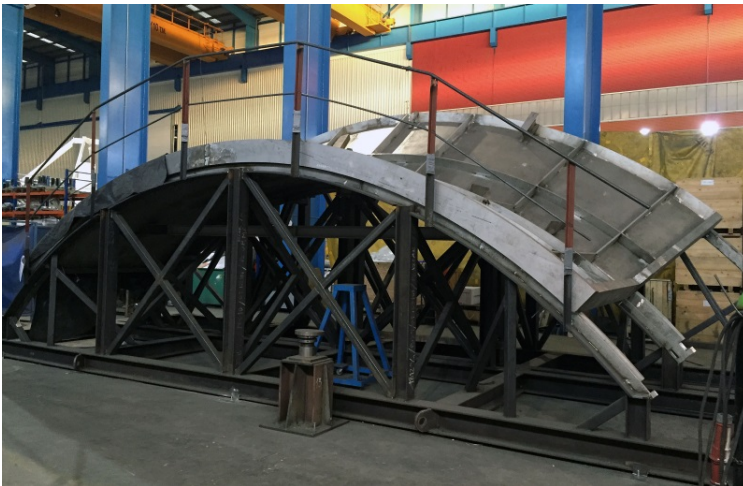
Upper part of sector 2-3 on the welding frames
