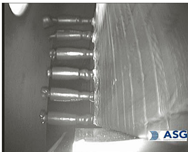
Helium inlet area of WP-02 under Paschen test
