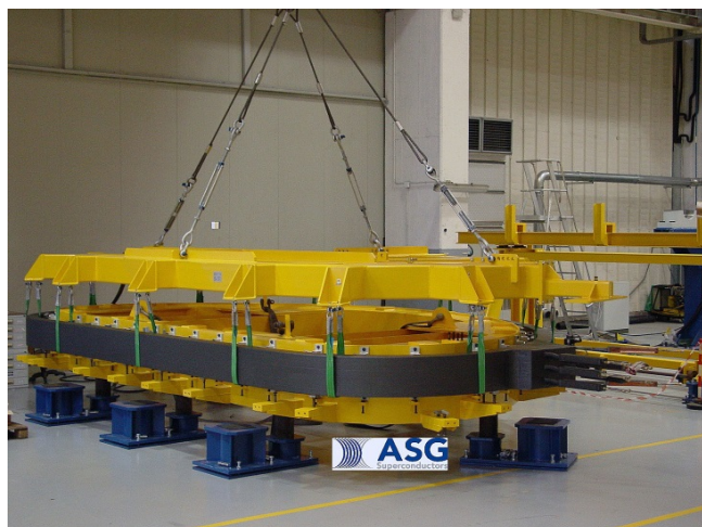
WP-01 placed on the tooling for case insertion
