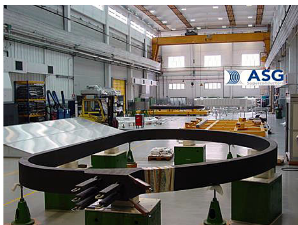
WP-02 during final dimensional tests
