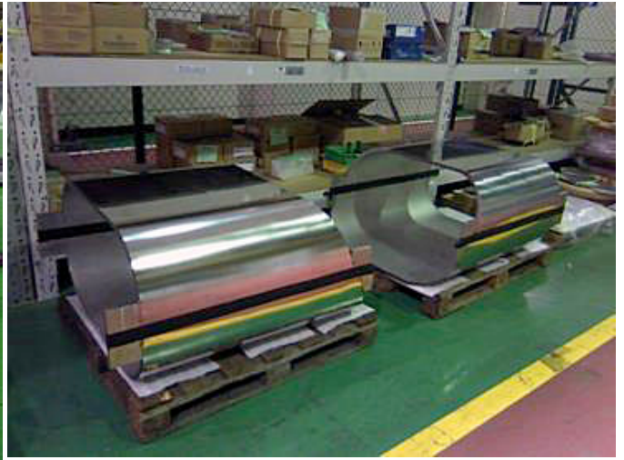
Figure 2: Horizontal port after bending
