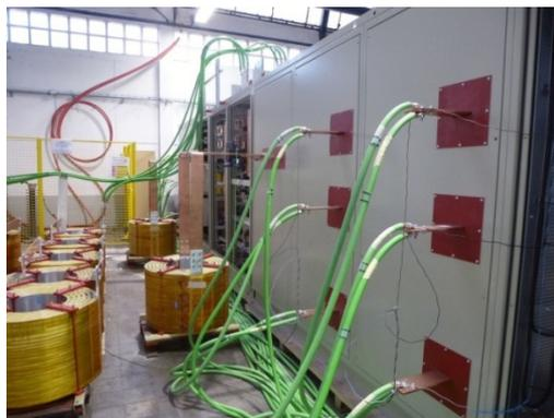
JEMA Laboratories, FPPC test hall, the rear view of FPPC converter connected to transformers
