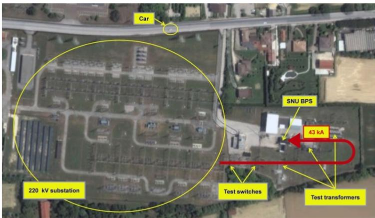
Figure 5: Set-up for the BPS electro-dynamic resistance test at 43 kA
