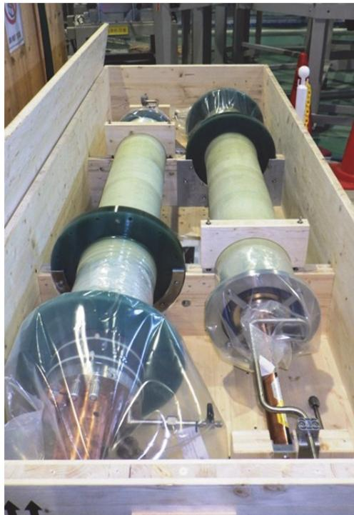
The pair of HTS CLs in a wooden box for transportation
