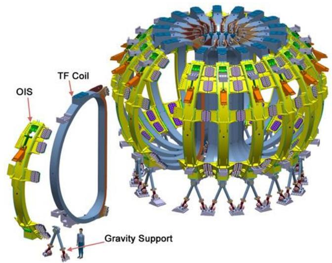
Figure 2: Final assembly of the TF coils (blue), OISs (yellow) and gravity supports (18 sets in total)
