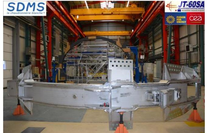
Figure 4: Pre-assembly tools for the TF coil and OIS
