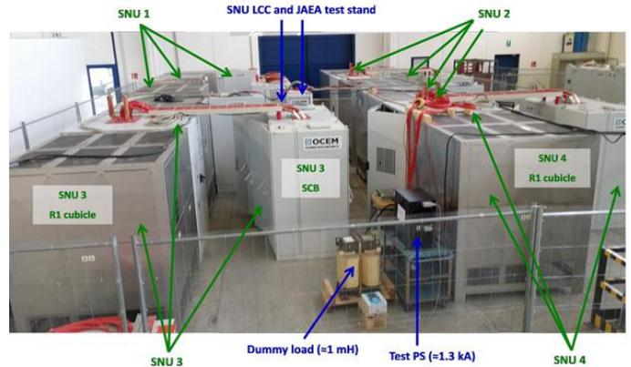
Figure 4: Complete SNU system set up for the routine tests
