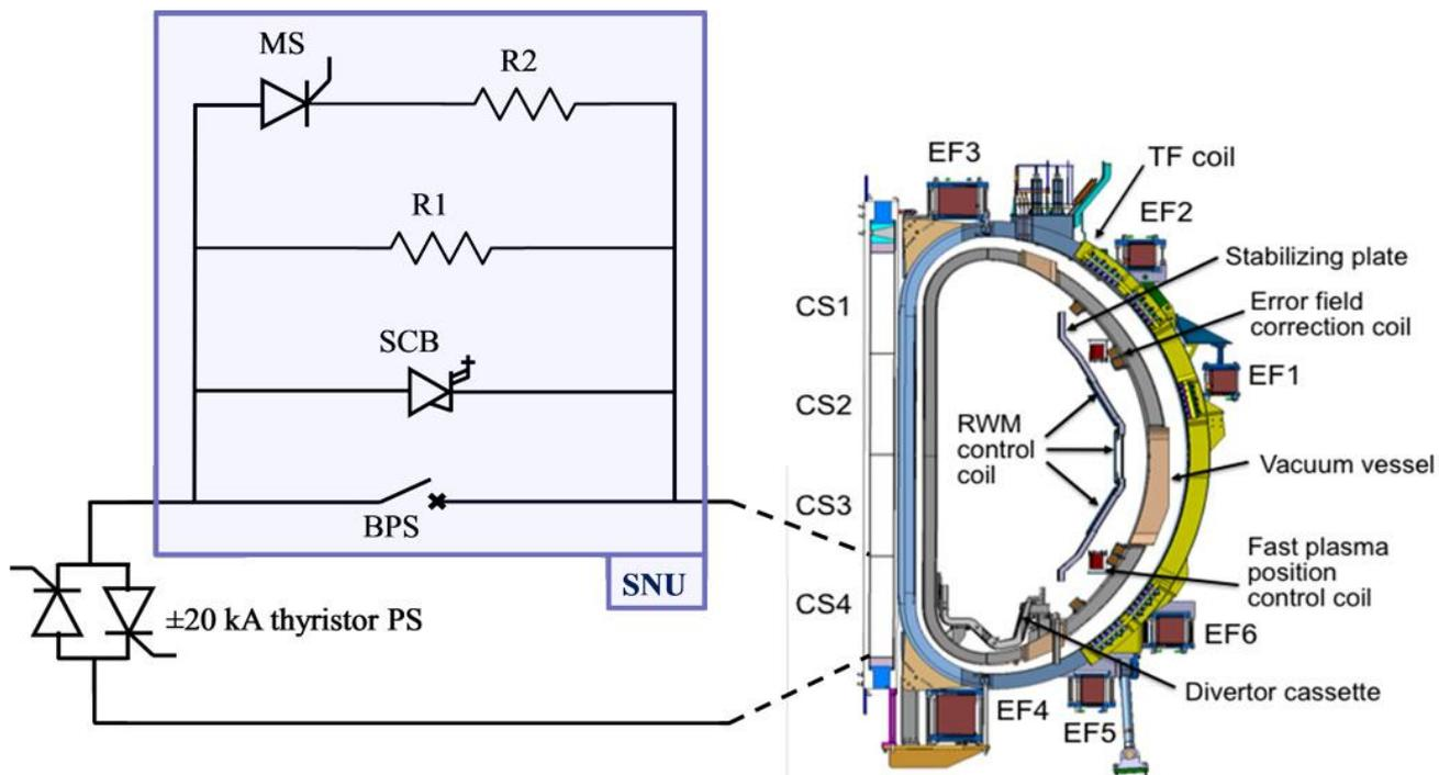
Figure 1: Simplified scheme of the SNU inserted in the CS module PS circuit
