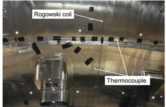
Figure 2: Rogowski coil and thermocouples
