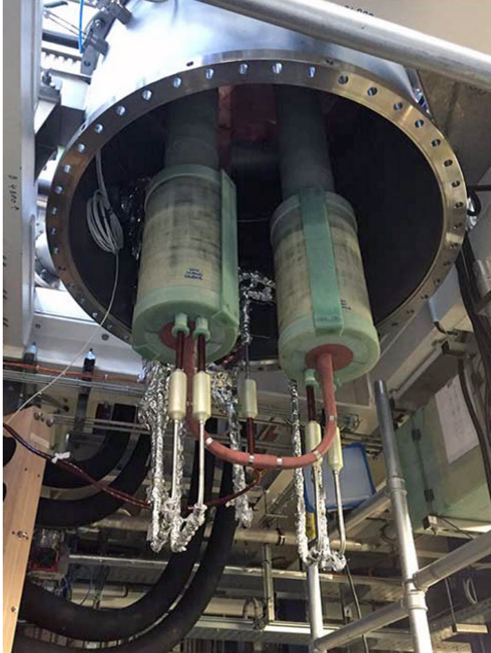
Figure 1: Installing the cold end of a HTS CL pair
