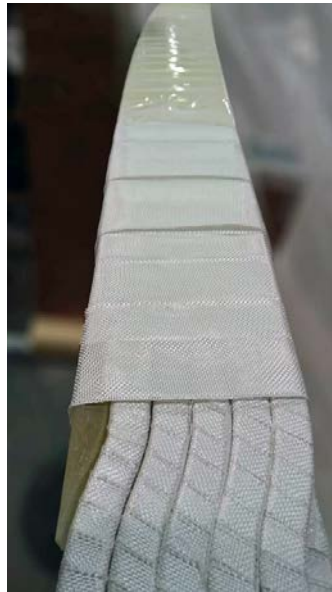
Figure 2: EFCC in the ground insulation overwrapping
