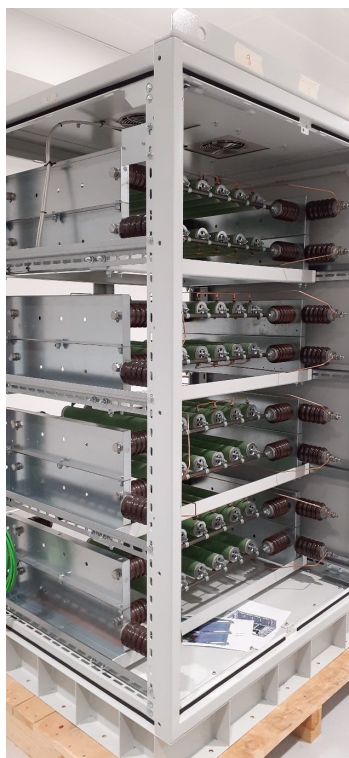
Figure 1: One AGS cubicle including the alternative grounding resistors for four poloidal coils, ready for factory tests
